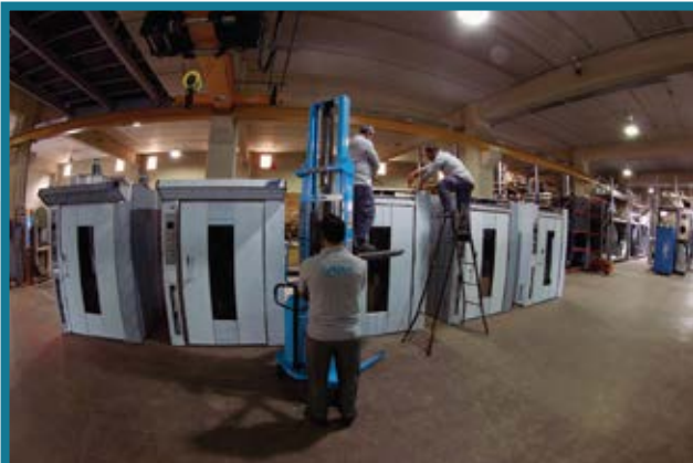
Ovens being assembled before getting shipped
